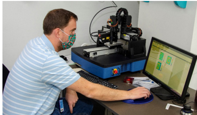
Product Quality Branch Chemist Joseph Piekarski uses a profilometer to measure heights of RTFs.
