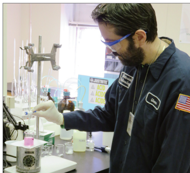
Chemist Glenn Flaim analyzing a wiping solution sample by acid titration method (left), and notes undergoing chemical rub testing (right).
