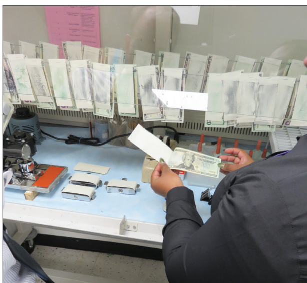
Chemist Glenn Flaim analyzing a wiping solution sample by acid titration method (left), and notes undergoing chemical rub testing (right).
