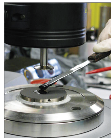
An ink viscosity test being performed using a rheometer in the BEP Quality Assurance Ink Laboratory.
