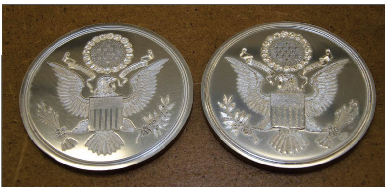
The finished counter and emboss Great Seal dies.
