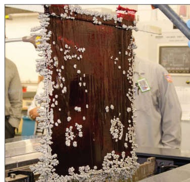
The nickel master in the nickel tank growing the 4-subject (Alto) counter plates.
