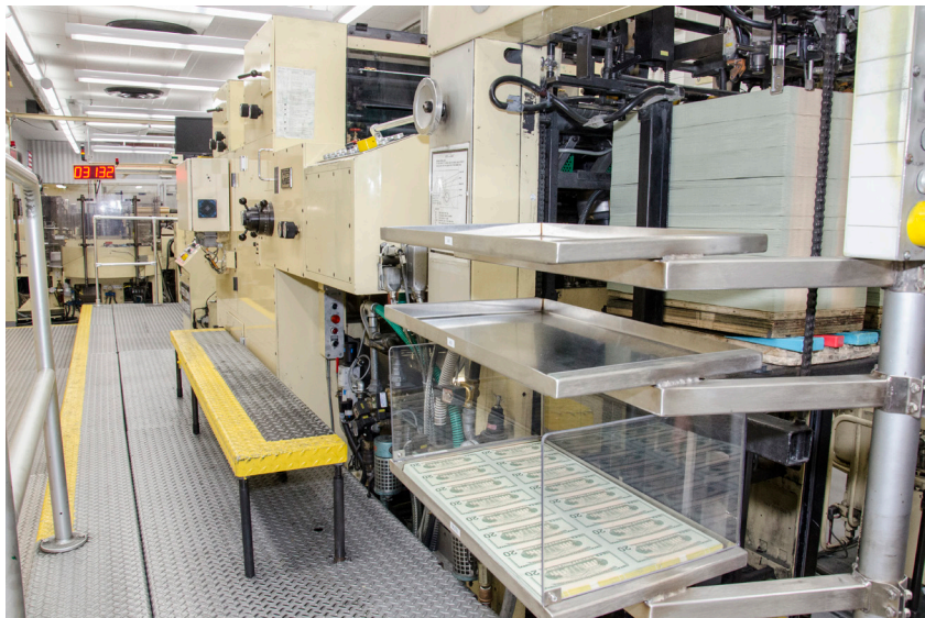
This is part of the Currency Overprinting and Processing Equipment that contains the feeder and printing unit. Sheets of currency are being accumulated for the printing of serial numbers, as well as both Treasury and Federal Reserve seals prior to being cut into single notes.
